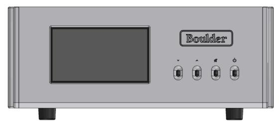
The 866 has a large, full-color display located on the left-hand side of the front panel. There are four buttons to control **Volume Up, Volume Down, Mute,** and **Standby** located on the right-hand side of the front panel.
