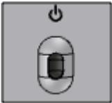
Pressing the Standby button will put the 812 into Standby mode. This will turn OFF all circuits except for the logic necessary to wake it up again.
