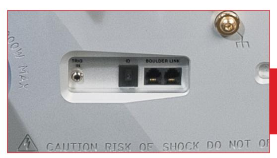
Boulder Link is a means of interconnecting Boulder products so that their microprocessors can talk to each other, pass important information, and issue commands. Among the key features, Boulder Link allows sequential initiation of power amplifiers and other products. Boulder power amplifiers can send messages to Boulder preamplifiers and shown on the preamplifier's display.
