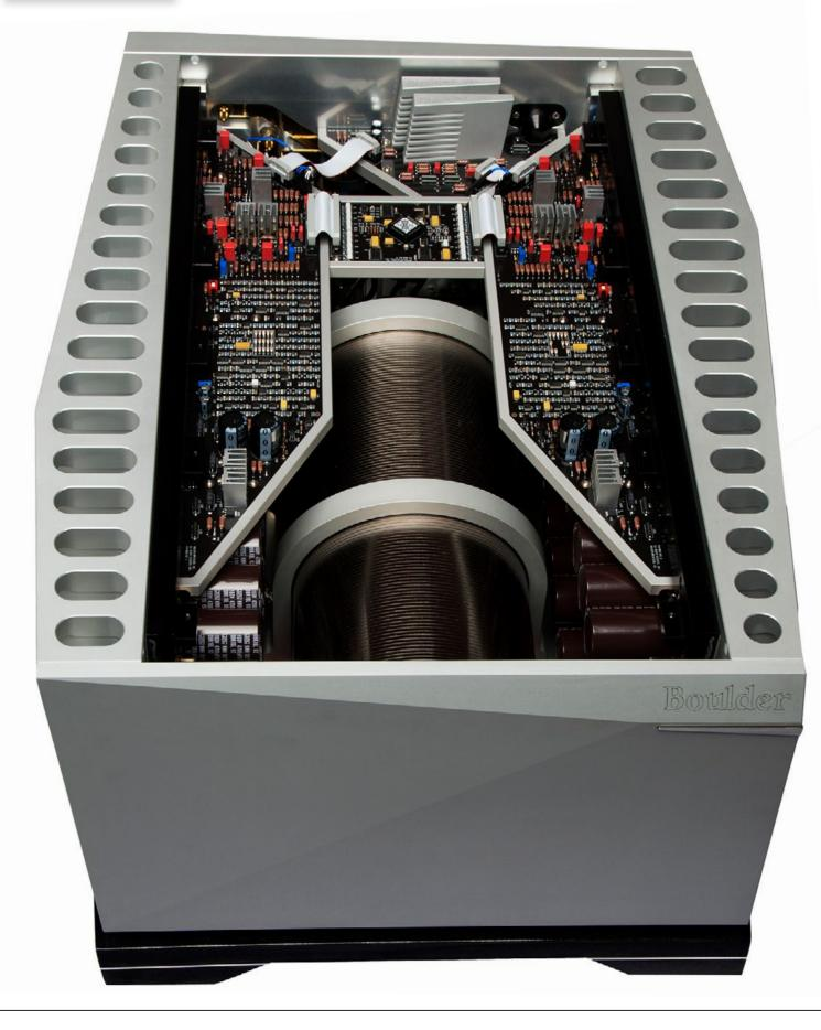
Fully balanced, differential power amplifiers from start to finish, the 3050s offer only balanced inputs, and the driver stage consists of Boulder's latest discrete 99H modules. A giant metal tunnel runs through the center of the amplifier chassis, with four separate, potted transformers inside, which helps drop all mechanical and electrical noise to the theoretical minimum.
