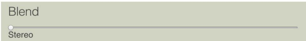
The **Blend Slider** adjusts the 3010's output from wide stereo separation to mono output. This may be useful when listening to recordings with images that are hard-panned to one channel or when listening to monaural phono recordings with a stereo phono cartridge. The Blend function is adjusted and indicated in decibels (dB).
