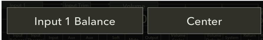
The screen will show a box reading **Input Balance** on the left side of the display and a box showing the Input Balance level on the right side of the screen. To adjust the Input Balance, rotate the **Center Control Knob** to the left or right until the desired balance offset is obtained as indicated in the display. A maximum of **12.0 dB** of offset may be programmed.
