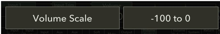
To adjust these features, press the **Volume Scale/Resolut.** button while in **Setup** mode. “**Volume Scale**” will show on the left side of the display along with a selection choice on the right. Rotate the **Center Control Knob** to the **right** (clockwise) to **increase** the display reading for maximum attenuation. Rotate the **Center Control Knob** to the **left** (counter-clockwise) to **decrease** the display reading for maximum attenuation.
