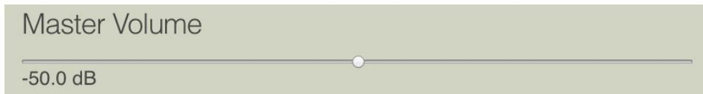
The **Master Volume Slider** adjusts the volume control and attenuation of the 3010. When adjusted, the Master Volume Slider will control the output of all three outputs simultaneously and has a range from **INF** (infinite attenuation) to **0.0 dB** (+20.0 dB of gain and maximum output). The volume control setting will appear under the left side of the Master Volume Slider.
