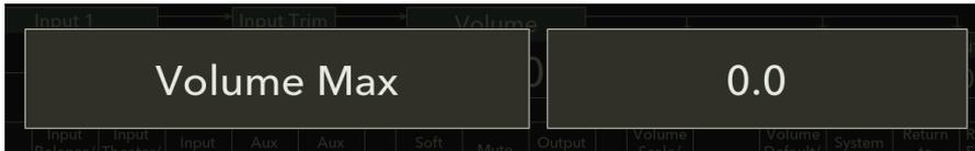
Once you have chosen a Volume Default setting, press any button on the front panel Button Bar. “**Volume Max**” will appear on the left side of the display along with a selection choice on the right. Rotate the **Center Control Knob** to select your desired maximum volume level. A Volume Max range from **-20.0 dB** to **0.0 dB** (no attenuation) is possible.
