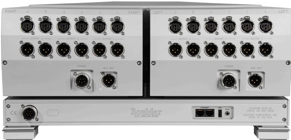
Connections from sources such as a CD player, DVD player, phono preamplifier, tuner, or cable/satellite receiver can be made to the analog input connections.
