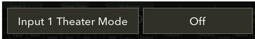
While in **Setup** mode, it is possible to program a specific input to be set to unity gain for use with a surround sound processor in a home cinema setting. Any of the 3010's inputs can be programmed to unity gain. This is called **Theater Mode**. When an input has been programmed for Theater Mode, the volume and balance controls will have no effect on volume or balance levels and the volume level must be controlled by the surround sound processor. “**UNITY**” will be shown in the display.
