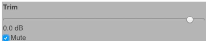
**Output Trim Sliders** for each output are shown in three boxes. These sliders allow you to make adjustments to the output level of each output relative to all others. For example, this may be useful when trying to even out the frequency response of the loudspeaker in a bi- or tri-amplified system.
