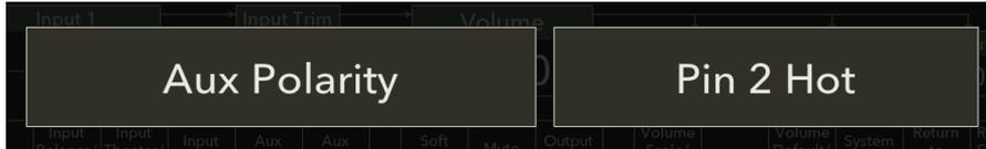
The polarity of the Auxiliary Output may also be adjusted to match the associated equipment used. All Boulder products adhere to the AES Standard of Pin-2 “Hot” or positive. Products which are configured for Pin-3 Hot operation are considered “polarity inverted.”
