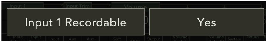
While in **Setup** mode, it is possible to program specific inputs so that they are recordable and the signal is routed to the Auxiliary output to prevent feedback loops. When in this mode, the input signal will not be affected by the volume control.
