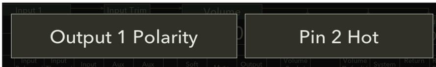
The polarity of each output can be configured individually in the Output Polarity screen. The Output Polarity is configured in successive screens, so Output 1 will have to be configured before Output 2, etc.
