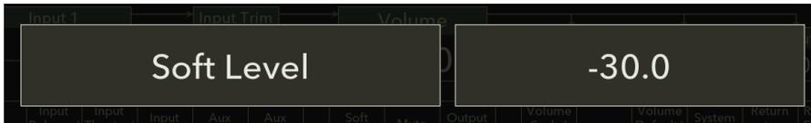
The Soft feature allows for temporary volume reduction without losing the original setting. The Soft Level will attenuate the current volume control setting by an additional amount from -6.0 dB to -80.0 dB as programmed into the Soft Level feature. Because personal use of this feature varies, the actual level of attenuation can be adjusted to suit your needs.
