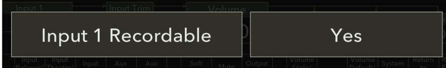
Instead of having hardware-dedicated inputs for playback (tape) monitors, any input may be chosen for this purpose through software selection. Connect the outputs of these recorders to any input you have chosen in the previous section.
