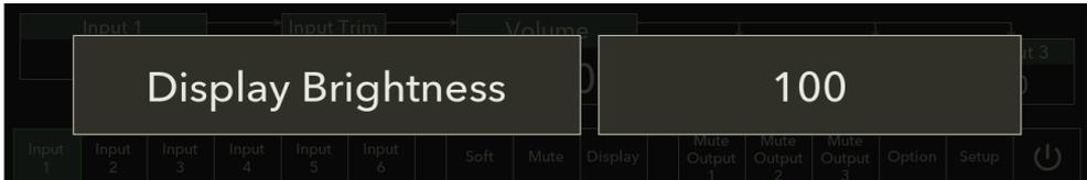
The brightness of the display can be adjusted as well as turning the display completely off. The **Display** setting determines the brightness of the display, from 0% (off) to 100% (full brightness).
