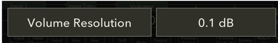
Once you have chosen a Volume Scale, press the any button on the front panel Button Bar. “**Volume Resolution**” will appear on the left side of the display along with a selection choice on the right. Rotate the **Center Control Knob** to select “**0.1 dB**”, “**0.5 dB**” (default), or “**1.0 dB**” per step as shown on the right side of the display.
