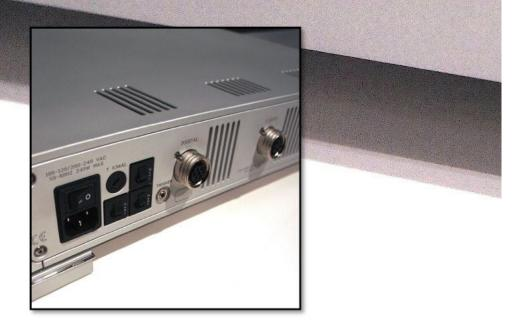
from emitting mechanical noise, a DC filter circuit blocks up to 3VDC on the AC mains. DC is one of the primary causes of transformer hum, thus this circuit is essential in order to maintain silent operation in any environment.
