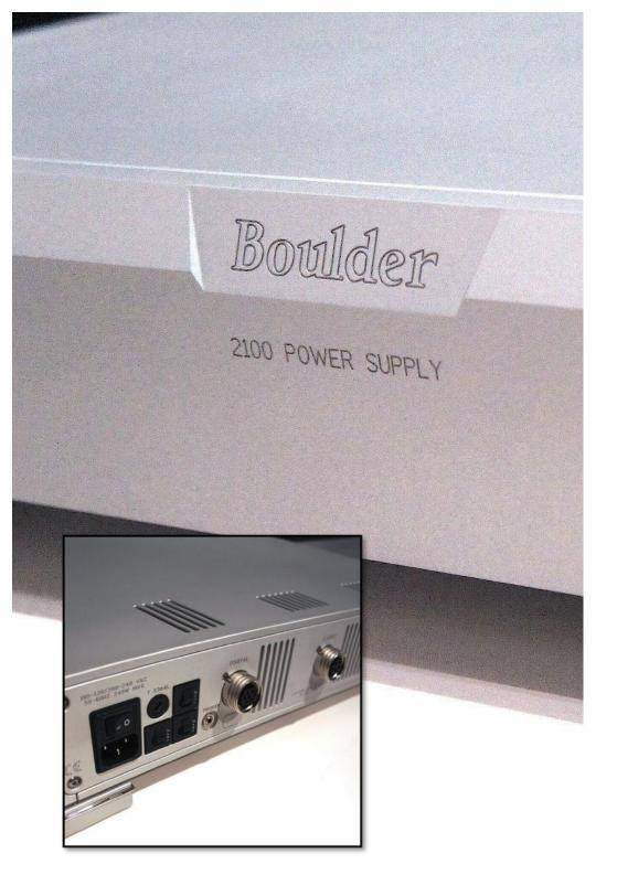
from emitting mechanical noise, a DC filter circuit blocks up to 3VDC on the AC mains. DC is one of the primary causes of transformer hum, thus this circuit is essential in order to maintain silent operation in any environment.
