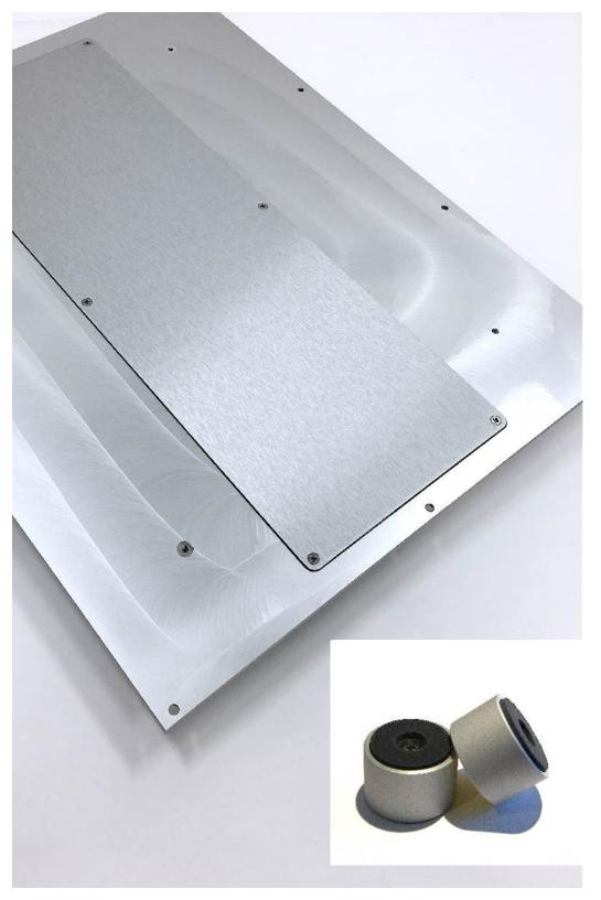
material compressed between the top cover and a stainless steel plate screwed to the underside of the cover. The layer of self-adhesive and elastic aircraft damping material is sandwiched between the top cover and stainless steel plate to form a complete constrained layer damping system itself rather than a plate with damping material attached to it. The top cover assembly is then bolted to the heatsinks, front panel, and rear panel to prevent any rattling or vibration when installed.
