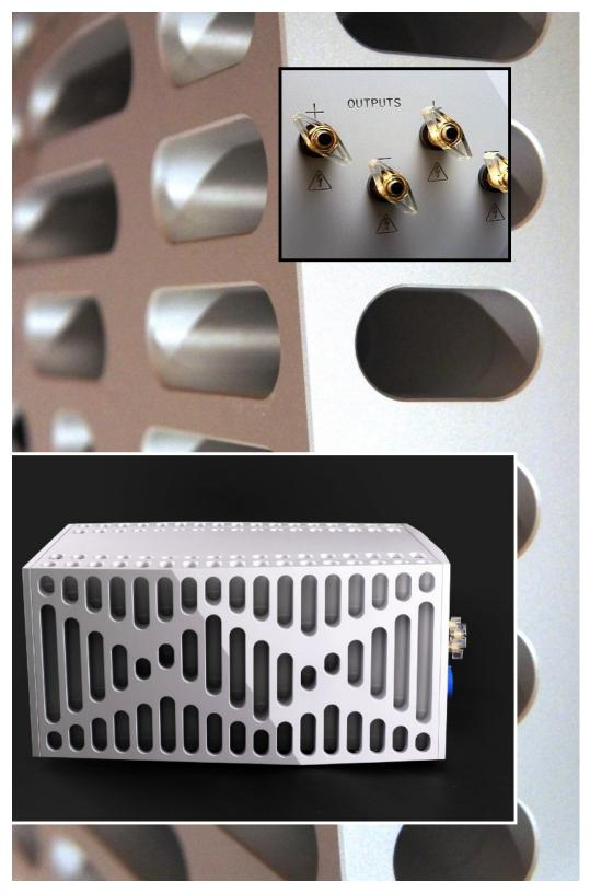
overall benefit of this methodology is that every output device operates at a uniform temperature due to the elimination of variance in clamping pressures that occur when each device is attached to a heatsink individually.
