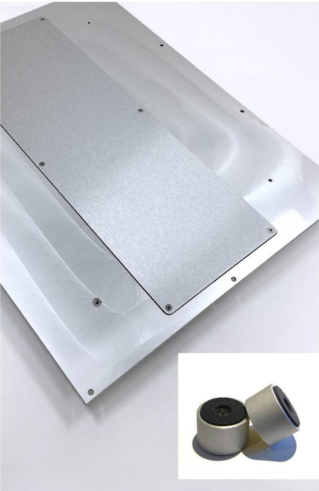
material compressed between the top cover and a stainless steel plate screwed to the underside of the cover. The layer of self-adhesive and elastic aircraft damping material is sandwiched between the top cover and stainless steel plate to form a complete constrained layer damping system itself rather than a plate with damping material attached to it. The top cover assembly is then bolted to the heatsinks, front panel, and rear panel to prevent any rattling or vibration when installed.
