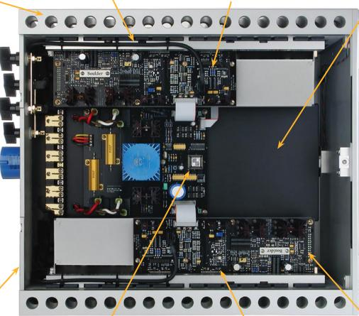
Boulderlink allows multiple 1050s to be sequentially turned on, and transmit their status to the display on a Boulder preamplifier Supervising microprocessor oversees all functions and communicates with other Boulders
